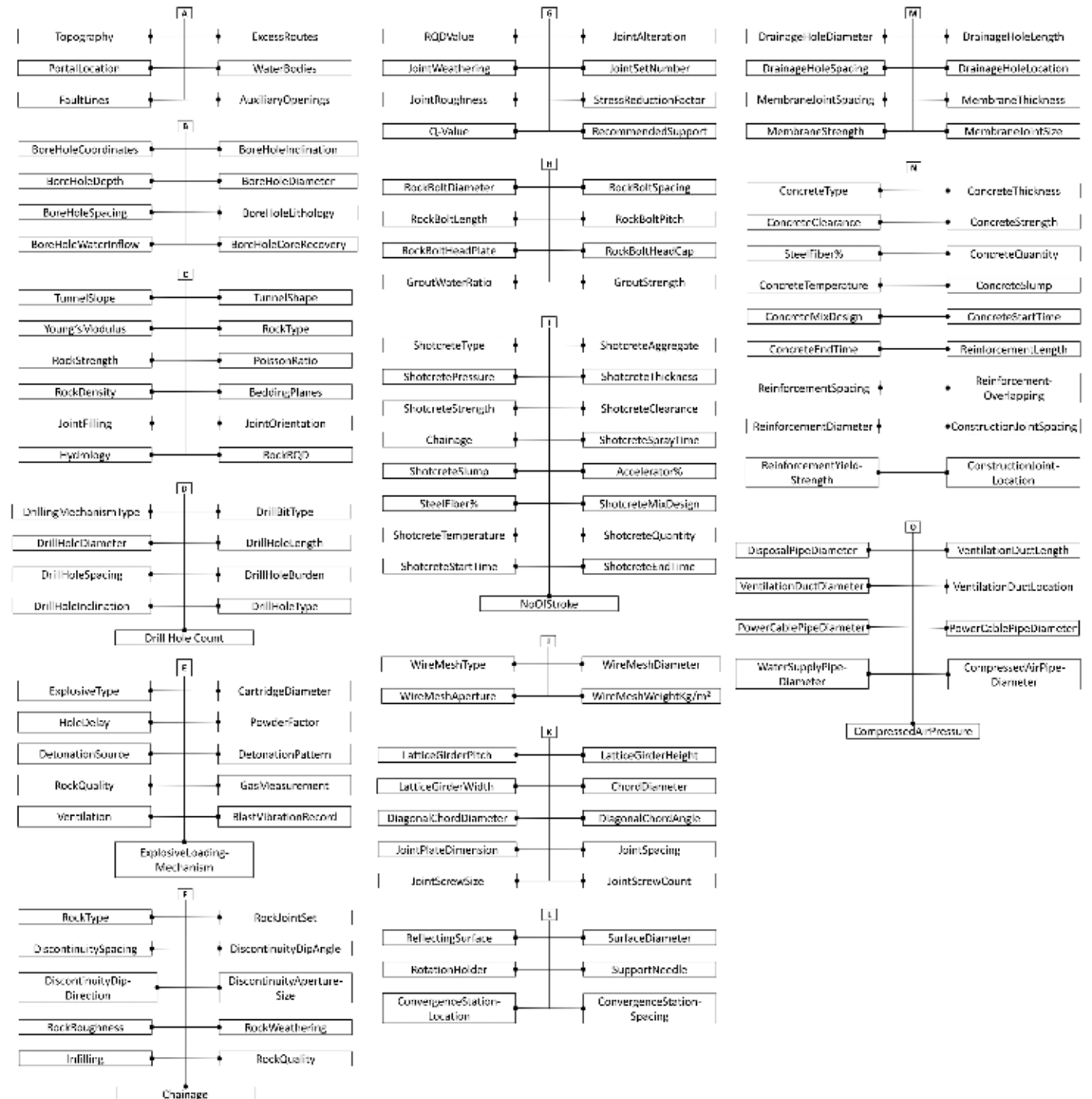
Fig. 15. Extract from the EXPRESS-G diagram of the IFC-based data model for drill-and-blast tunnel construction.
