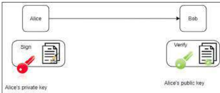
Fig. 1. Public key digital signature scheme: Alice uses her private key to sign her messages. Bob can verify that the message was signed by Alice using Alice's public key.
