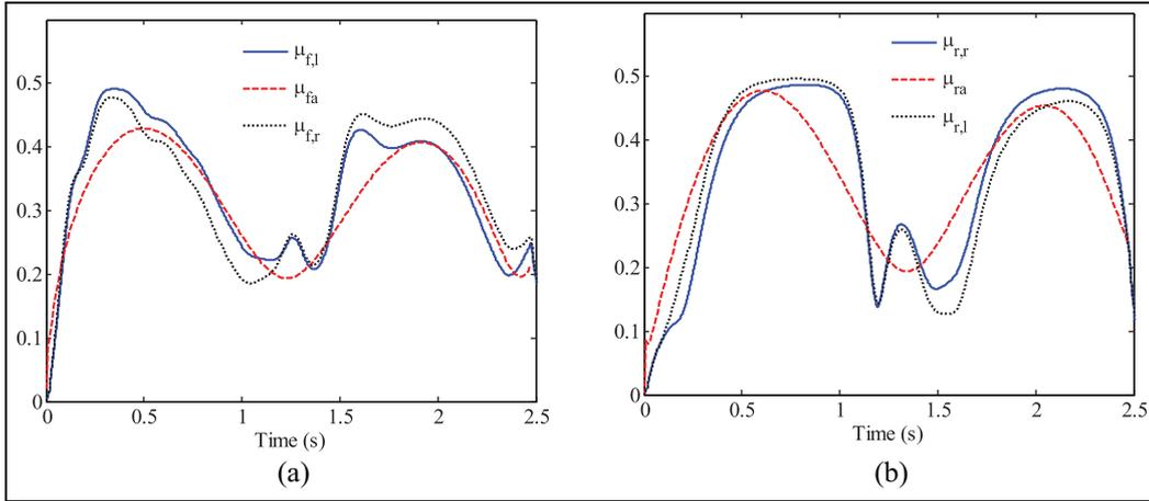
**Figure 7.** Comparison of approximate average friction coefficients and tyre friction coefficients: (a) Front tyres and (b) rear tyres.
