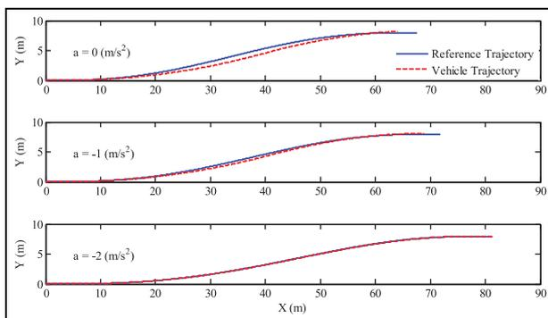
**Figure 12.** Reference and vehicle trajectories for complex scenario.
