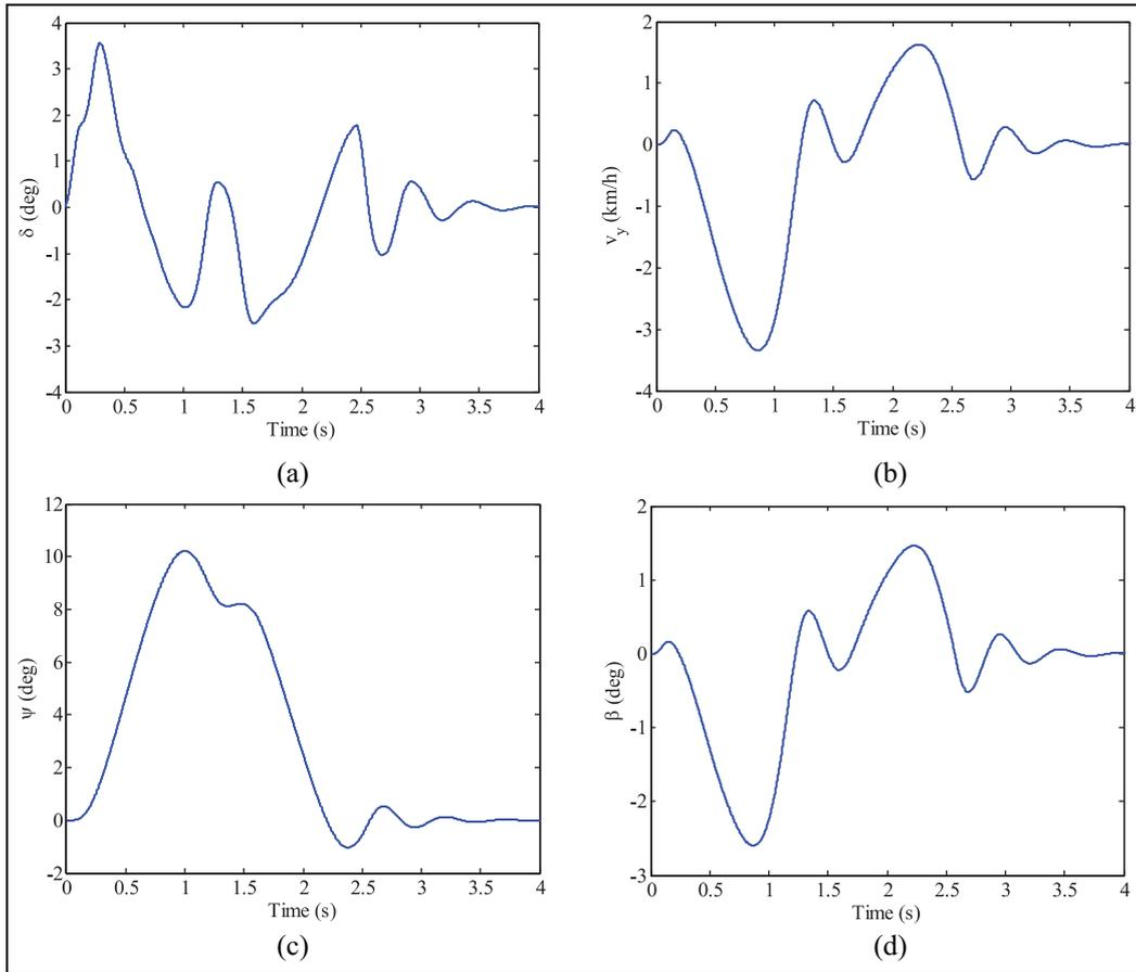
**Figure 10.** Lateral control: (a) Front-wheel steering angle, (b) lateral speed, (c) heading angle and (d) side-slip angle.
