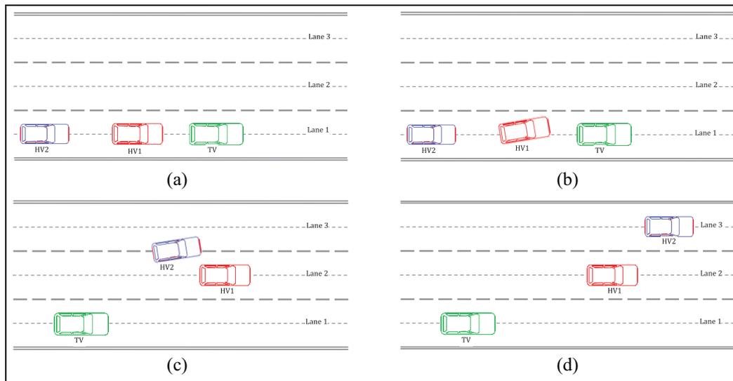
**Figure 11.** Complex scenario: (a) initial vehicle positions, (b) start of the manoeuvre, (c) moment that HV2 reaches to HV1 and (d) the end of manoeuvre.
