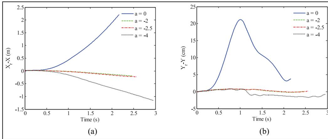
Figure 6. Tracking errors for all trajectories: (a) Longitudinal position error and (b) lateral position error.
