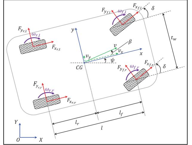
**Figure 3.** Seven degree of freedom vehicle model.
