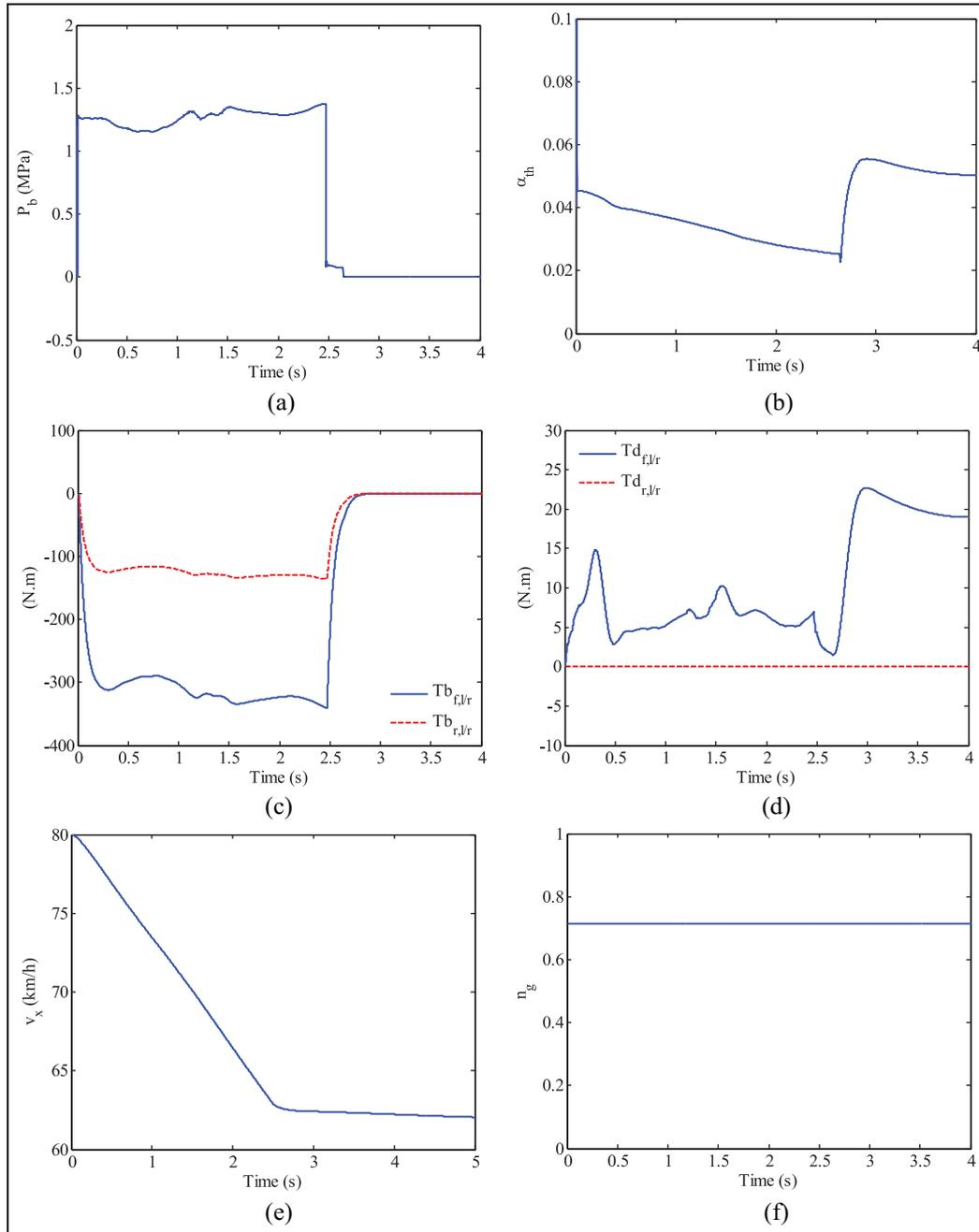
**Figure 9.** Longitudinal control: (a) Brake master cylinder pressure, (b) throttle opening, (c) wheel braking torques, (d) wheel driving torques, (e) longitudinal speed and (f) transmission gear ratio.
