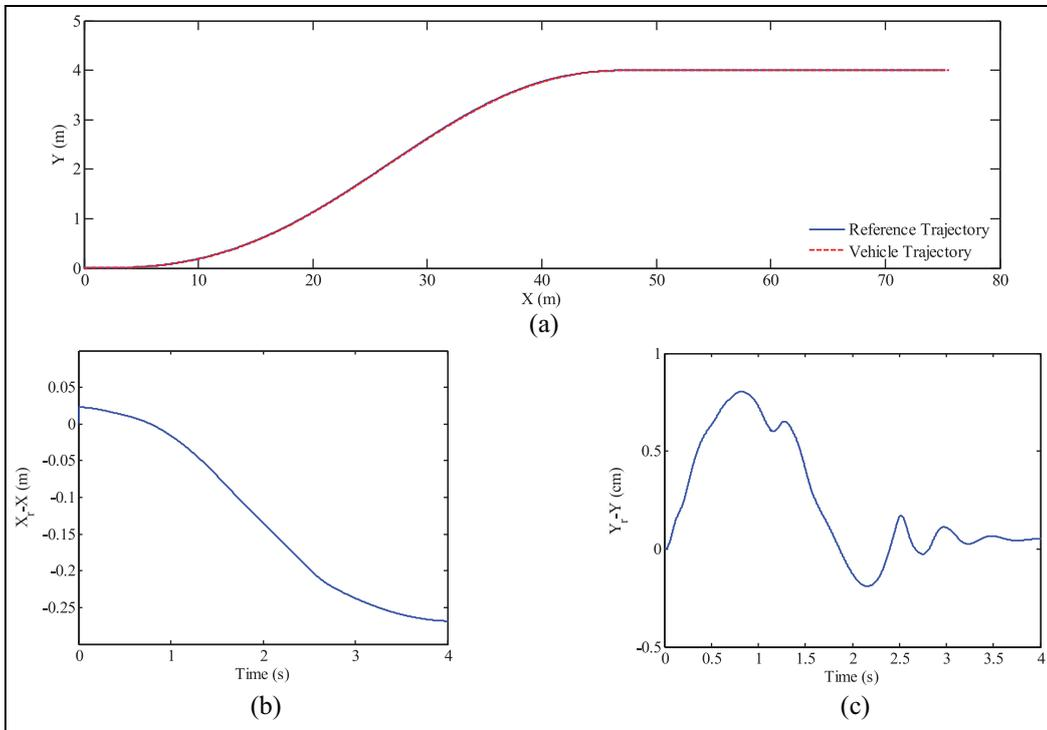
**Figure 8.** Overall performance of the combined controller: (a) Reference and vehicle trajectories, (b) longitudinal position error and (c) lateral position error.
