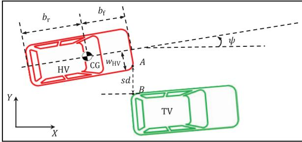
**Figure 4.** Description of the lateral distance between the HV and the TV.
