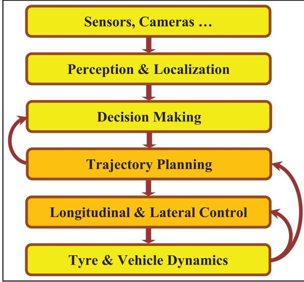
**Figure 1.** General architecture of a longitudinal and lateral guidance system.
