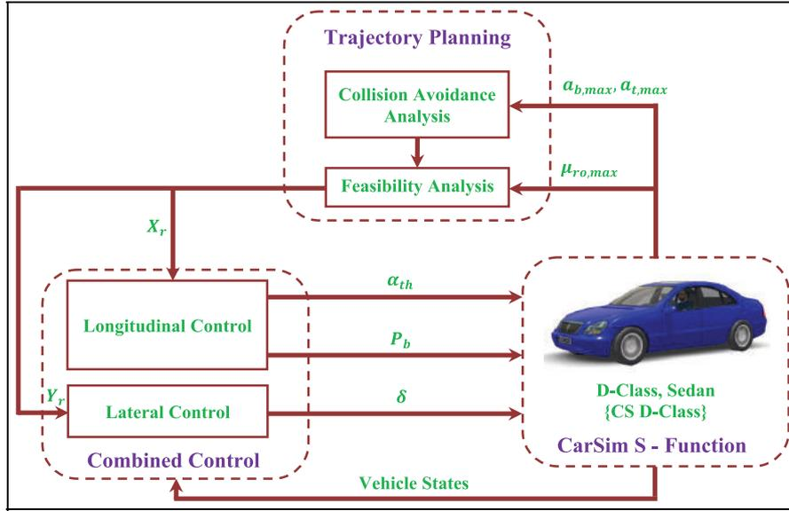
Figure 5. The block diagram of the combined longitudinal and lateral guidance system.
