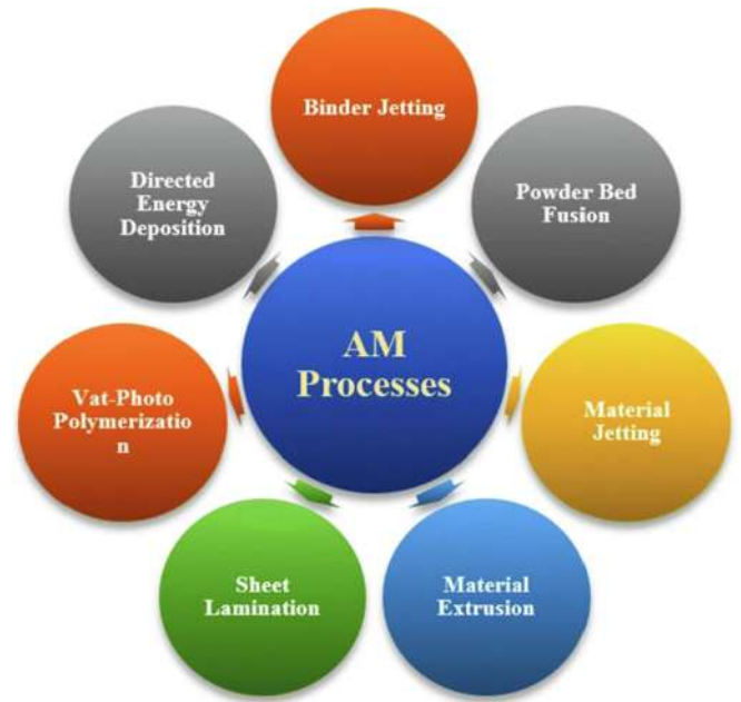
Fig. 2. Classification of Additive manufacturing.
