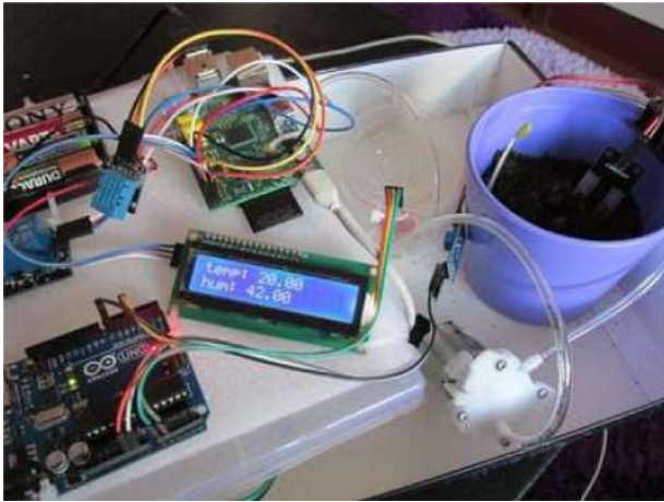
Fig. 4. Developed model of smart water quality monitoring system.
