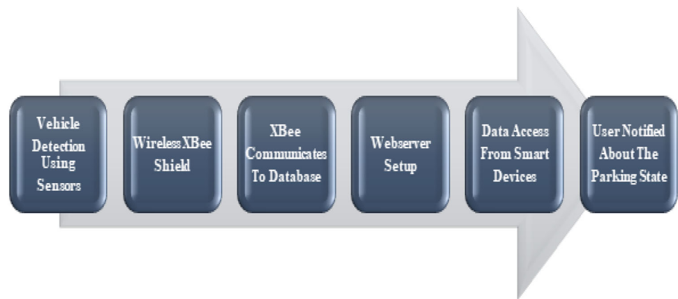
Fig. 8 Process flow diagram for the parking assistance system [59]
